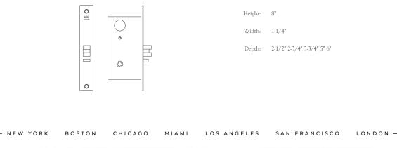
finishes are available. This lock is UL Listed and has a 3 hour fire rating.
